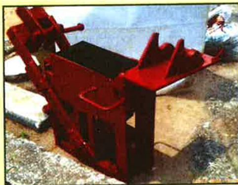
BCC/01/ V.S. CINVA RAM PRESS (MULTI-PURPOSE). SINGLE. BRICKSIZE: 290mm x 140mm
