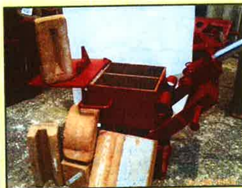
BCC/02/BOLYN DOUBLE BRICK PRESS (MULTI-PURPOSE) DOUBLE BRICK SIZE: 2NOS x 290mm x 140mm x 100m
