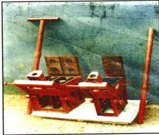
BOLYN DOUBLE INTERLOCKING BRICK PRESS, LIQUID MORTAR
