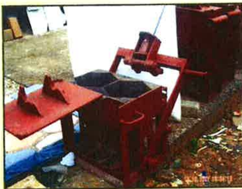
BCC/07/ BOLYN PAVING BRICK PRESS P.HEXA (HEXA PAVER).
