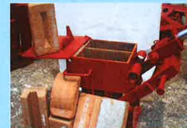
BCC/02/ BOLYN DOUBLE BRICK PRESS (MULTI-PURPOSE) DOUBLE BRICK SIZE: 2 NOS X 290MM X 140MM X 100MM.
