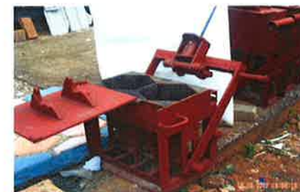
BCC/07/ PHEXA. BOLYN PAVING BRICK PRESS II. (HEXA PAVER).
