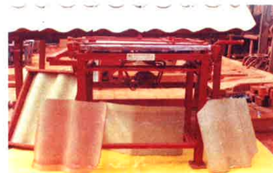
BCC/13 BOLYN-SUPER SEMI - ROOFING SHEET VIBRATION TABLE.
