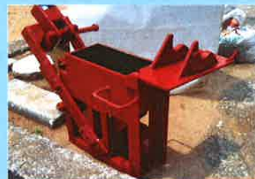
BCC/01/ V.S. CINVA RAM PRESS (MULTI-PURPOSE) SINGLE BRICK SIZE: 290MM X 140MM X 100MM
