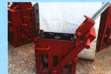
BCC/04/ BOLYN INTERLOCKING BRICK PRESS AFTER AIT, THAILAND (MODEL) INT(Thai) LIQUID MORTAR IN VERTICAL HOLES. BRICK SIZE: 300MM X 150MM X 100MM.
