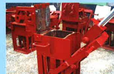
BCC/05/ BOLYN INTERLOCKING BRICK PRESS. NO MORTAR JOINT. BRICK SIZE: 230MM X 115MM X 120MM-Half Brick. or 230mm X 230mm X 120mm
